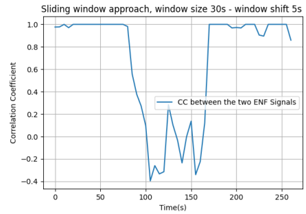
Fig. 6. CC obtained with the sliding window approach for a window size of 30s and a window shift of 5s.
