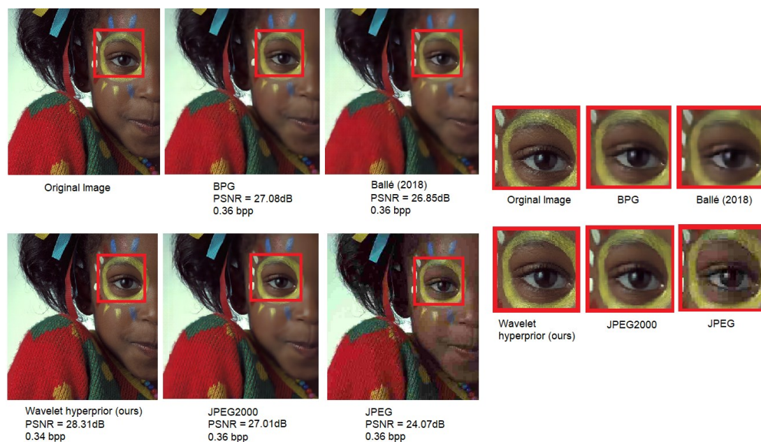
Fig. 4. At similar bit rates, our wavelet hyperprior method provides the highest visual quality on the Kodak dataset
